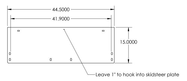
Flat blank bolt-on plate (Blank plate bolts into existing skid steer plate)
