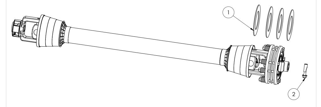
Replacement liner disks for the slip clutch, and lock bolts are available from Baumalight as wear parts. Otherwise, only complete PTO shafts are stocked.
