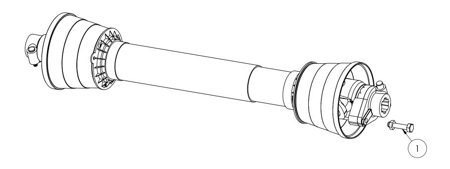
Replacement shear pins are available from Baumalight as wear parts. 5-packs are also available under part number D001646. Otherwise, only complete PTO shafts are stocked.
