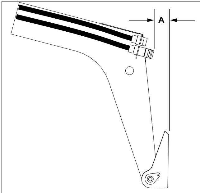
The distance (A) between the hydraulic couplers and the skidsteer quick attach plate should be at least 15.79 in. (401 mm).
