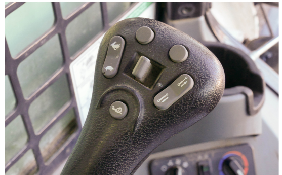
Control lever with auxiliary control switch.
