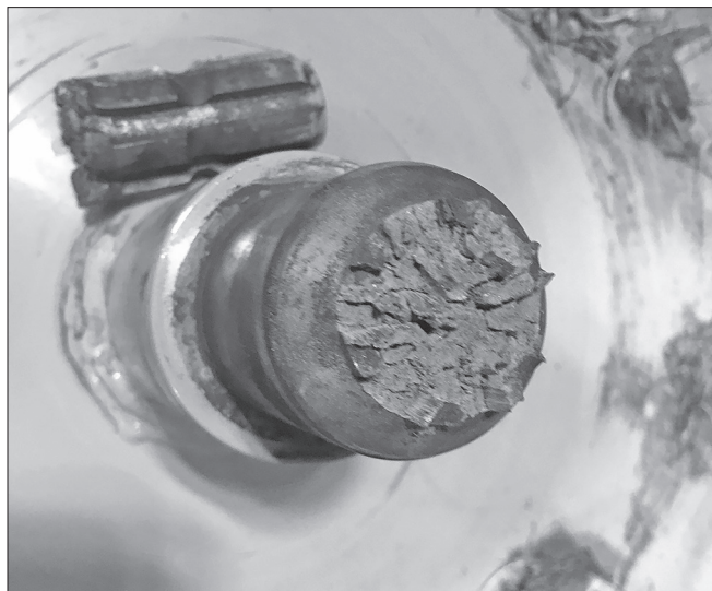
Broken Shaft From Severe Driveshaft Angle
