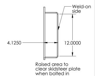
Blank weld on plate to bolt into Tree Spade
